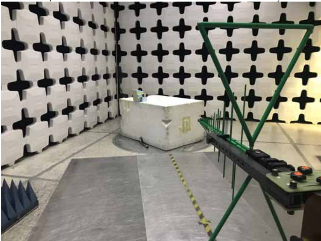
Test Setup for Radiated Emissions 30MHz to 1GHz – Vertical Polarity - Duck
