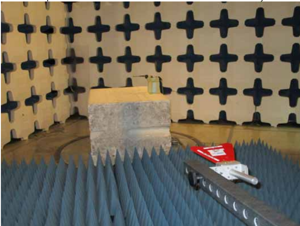
Test Setup for Radiated Rx Emissions Above 1GHz – Vertical Polarity - Duck
