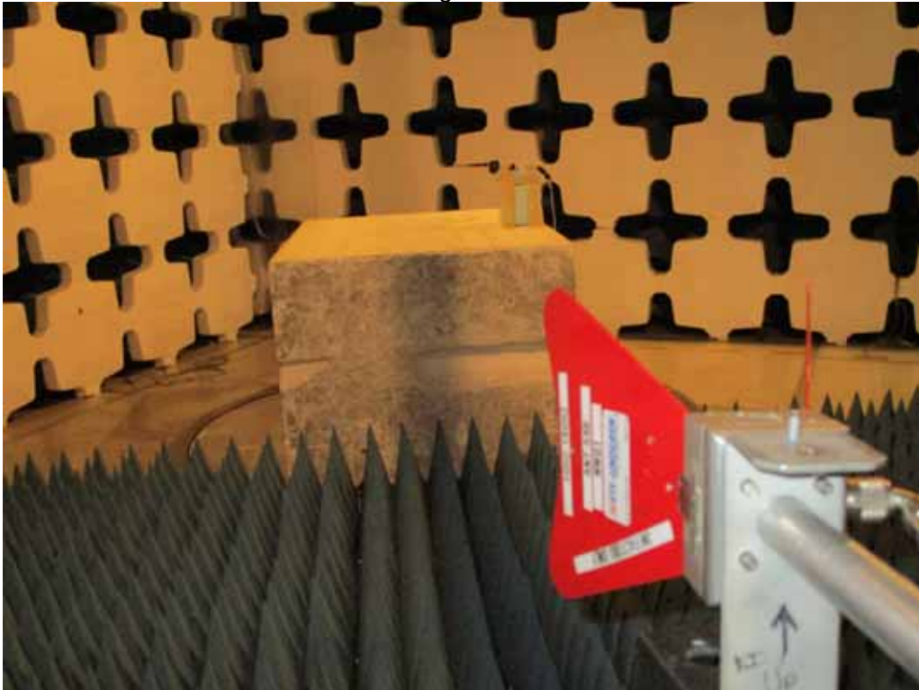
Test Setup for Radiated Rx Emissions Above 1GHz – Horizontal Polarity - Duck
