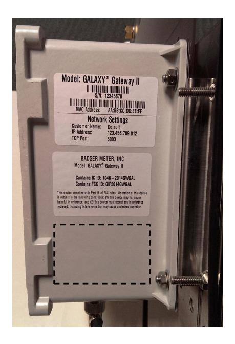
The third label will be installed based on which backhaul network is used. In LAN only configuration, there will not be a third label.
