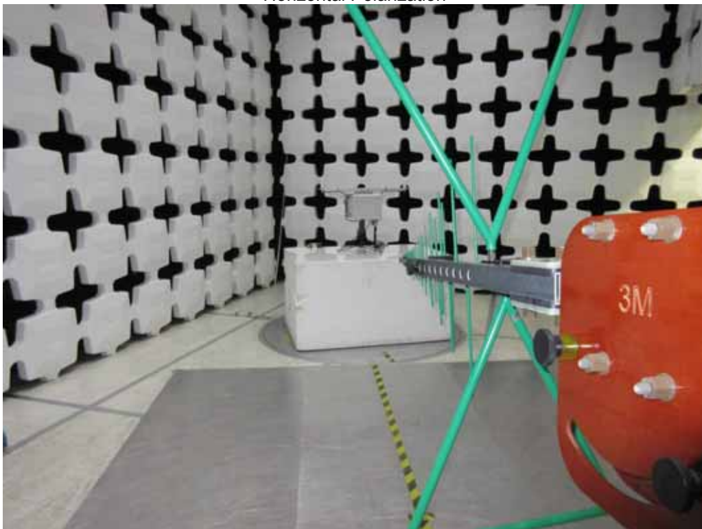
Test Setup for Radiated Emissions (Emerson Power Supply), 30MHz to 1GHz – Vertical Polarization
