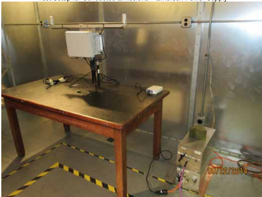
Test Setup for Conducted Emissions – Power over Ethernet (PoE)
