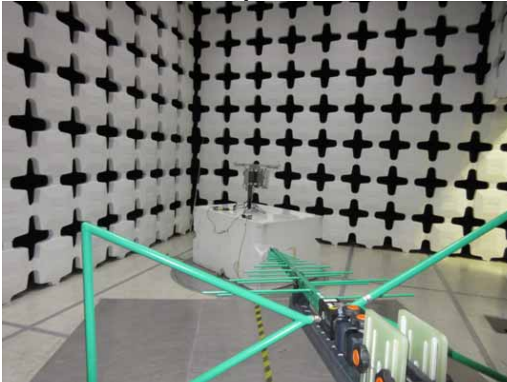
Test Setup for Radiated Emissions (Emerson Power Supply), 30MHz to 1GHz – Horizontal Polarization
