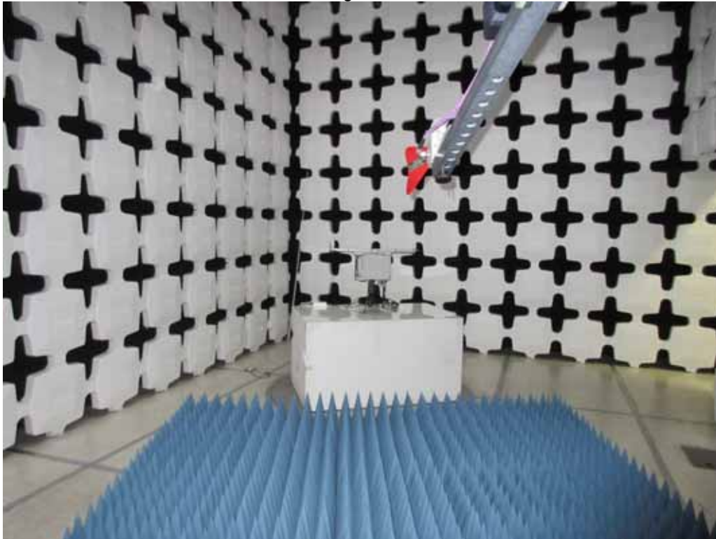
Test Setup for Radiated Emissions (Power over Ethernet), 1GHz to 10GHz – Horizontal Polarization
