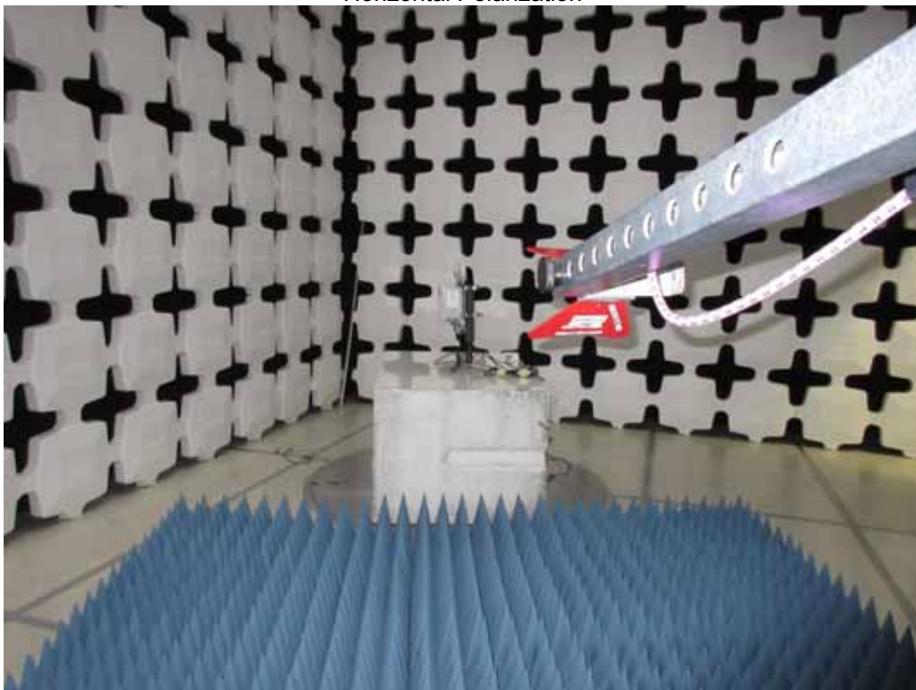
Test Setup for Radiated Emissions (Power over Ethernet), 1GHz to 10GHz – Vertical Polarization
