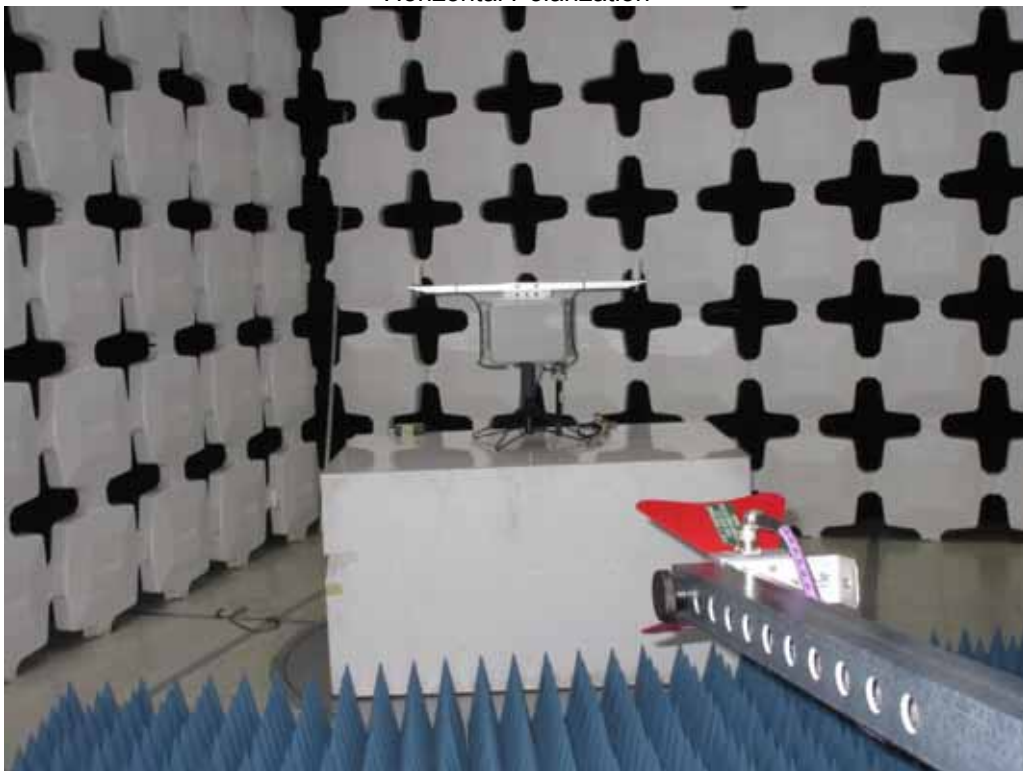
Test Setup for Radiated Emissions (Emerson Power Supply), 1GHz to 10GHz – Vertical Polarization
