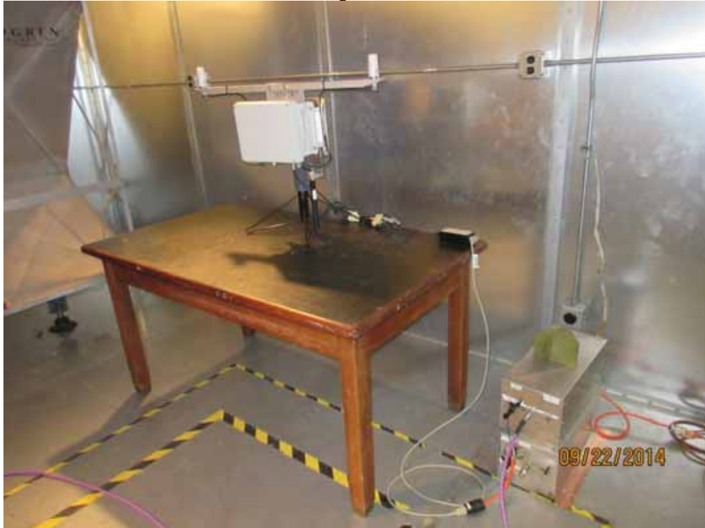
Test Setup for Conducted Emissions – Emerson Power Supply
