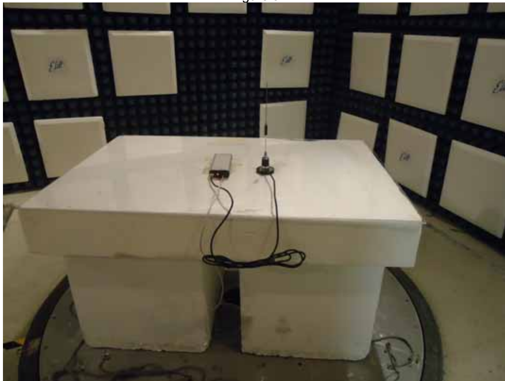
Test Setup for Radiated Emissions
