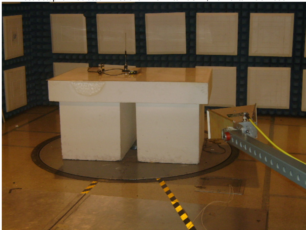
Test Setup for Radiated Emissions – 1GHz to 10GHz, Vertical Polarization
