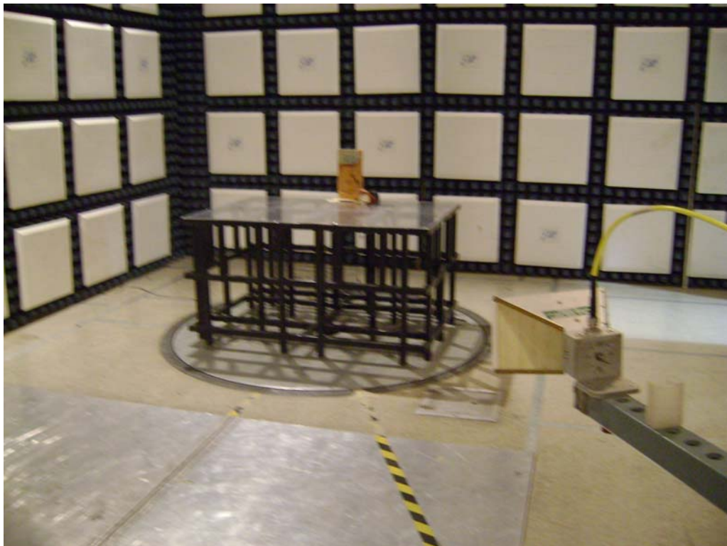
Test Set-up for Radiated Emissions, 1000-5000MHz - Vertical Polarization
