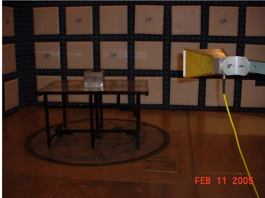
TEST SETUP FOR MEASUREMENT OF RADIATED EMISSIONS, HORIZONTAL POLARIZATION
