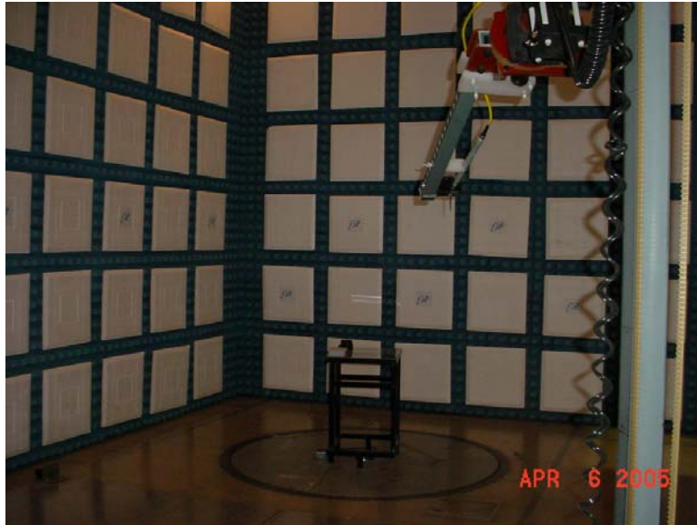
TEST SETUP FOR MEASUREMENT OF RADIATED EMISSIONS, VERTICAL POLARIZATION
