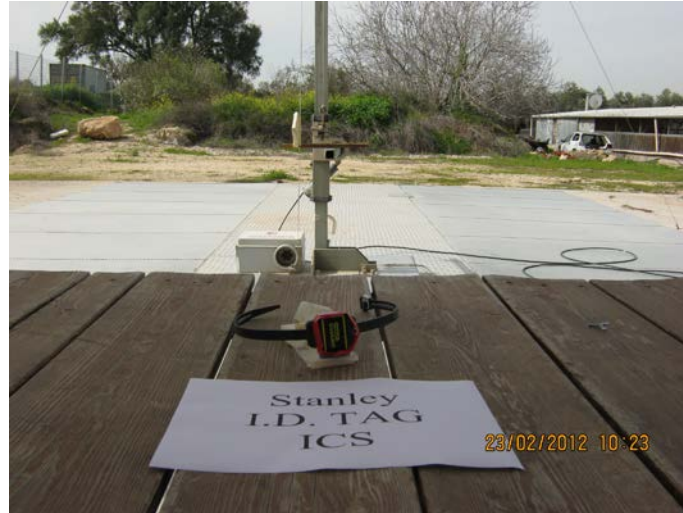
Figure 2 - Radiated Emission Test
