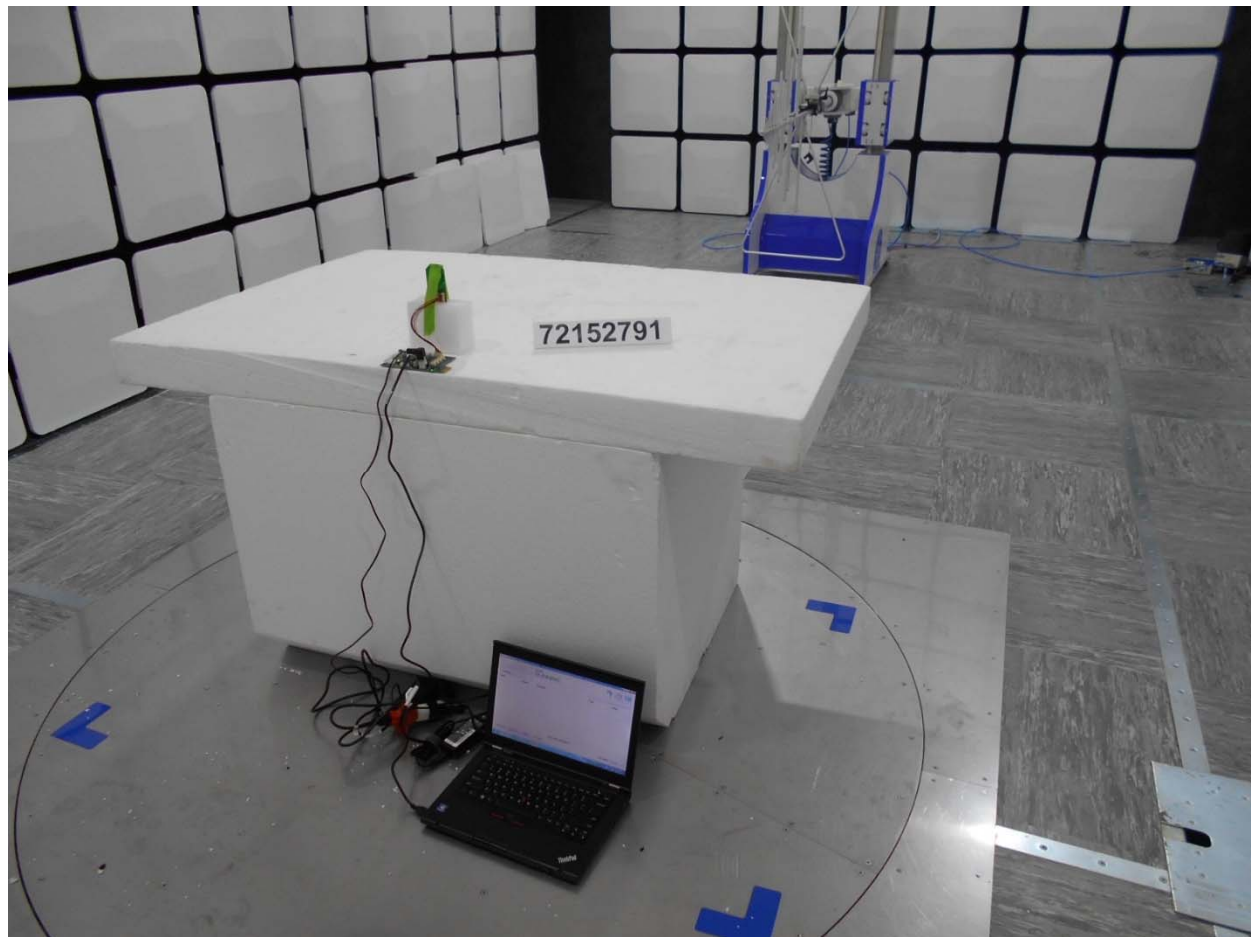
Photo 2.5.8-2 – Rear View of the Test Setup - Out of band emissions 30 - 1000MHz
