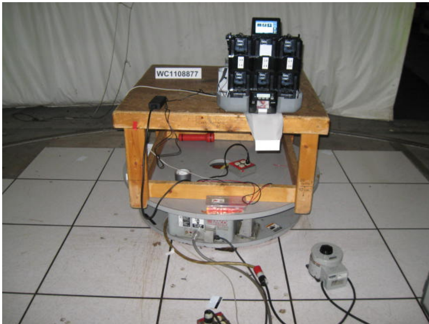
Test-setup photo(s): Radiated Emissions 30 - 1000 MHz
