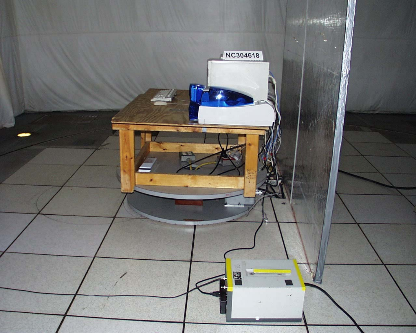
Test-setup photo(s): Conducted emission 150 kHz - 30 MHz
