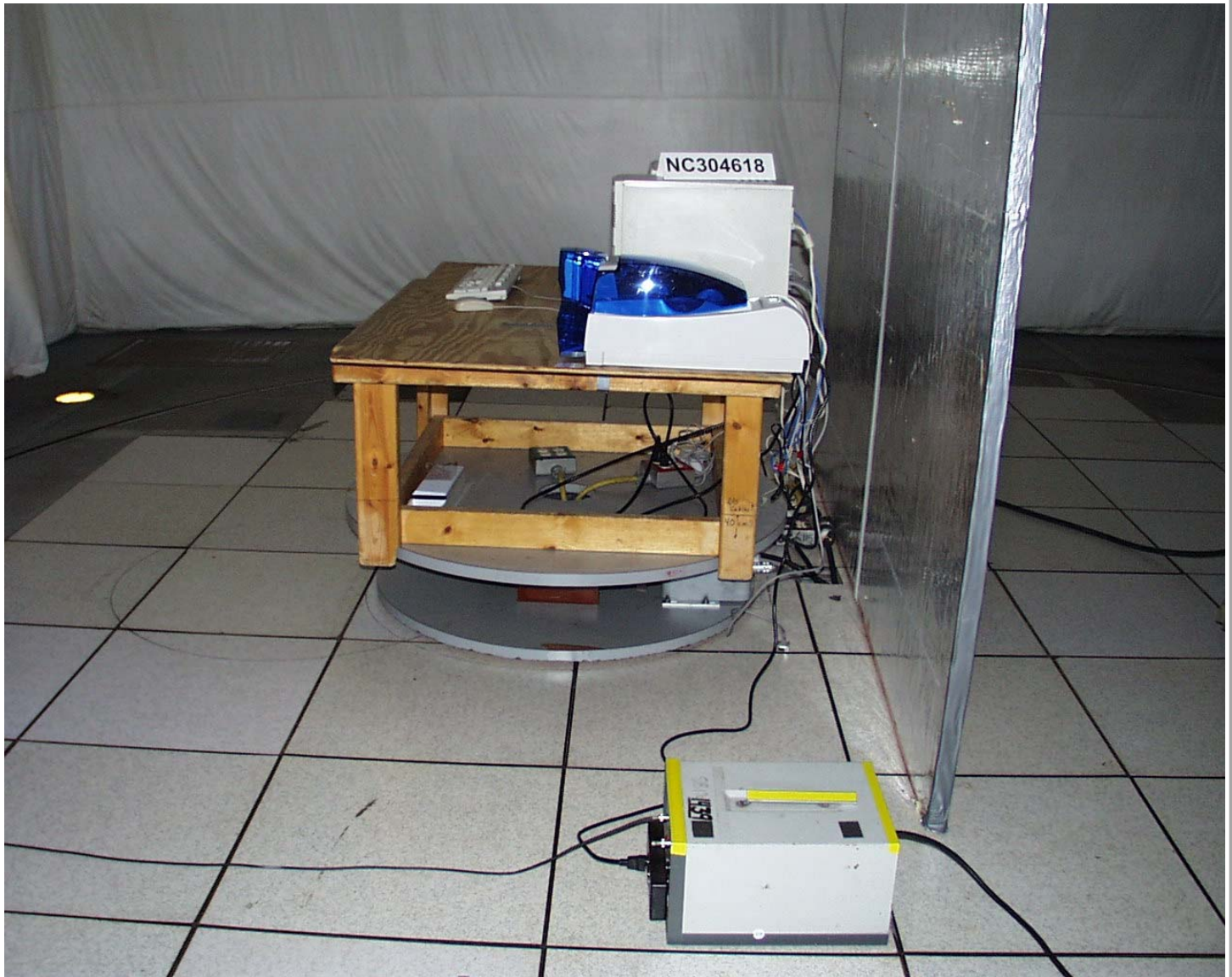
Test-setup photo(s): Conducted emission 150 kHz - 30 MHz
