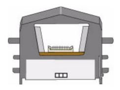
Do not touch the printing edge of the printhead in the printhead cartridge. If you do, use the cleaning pen to clean it. See Cleaning the printhead for steps to follow.
