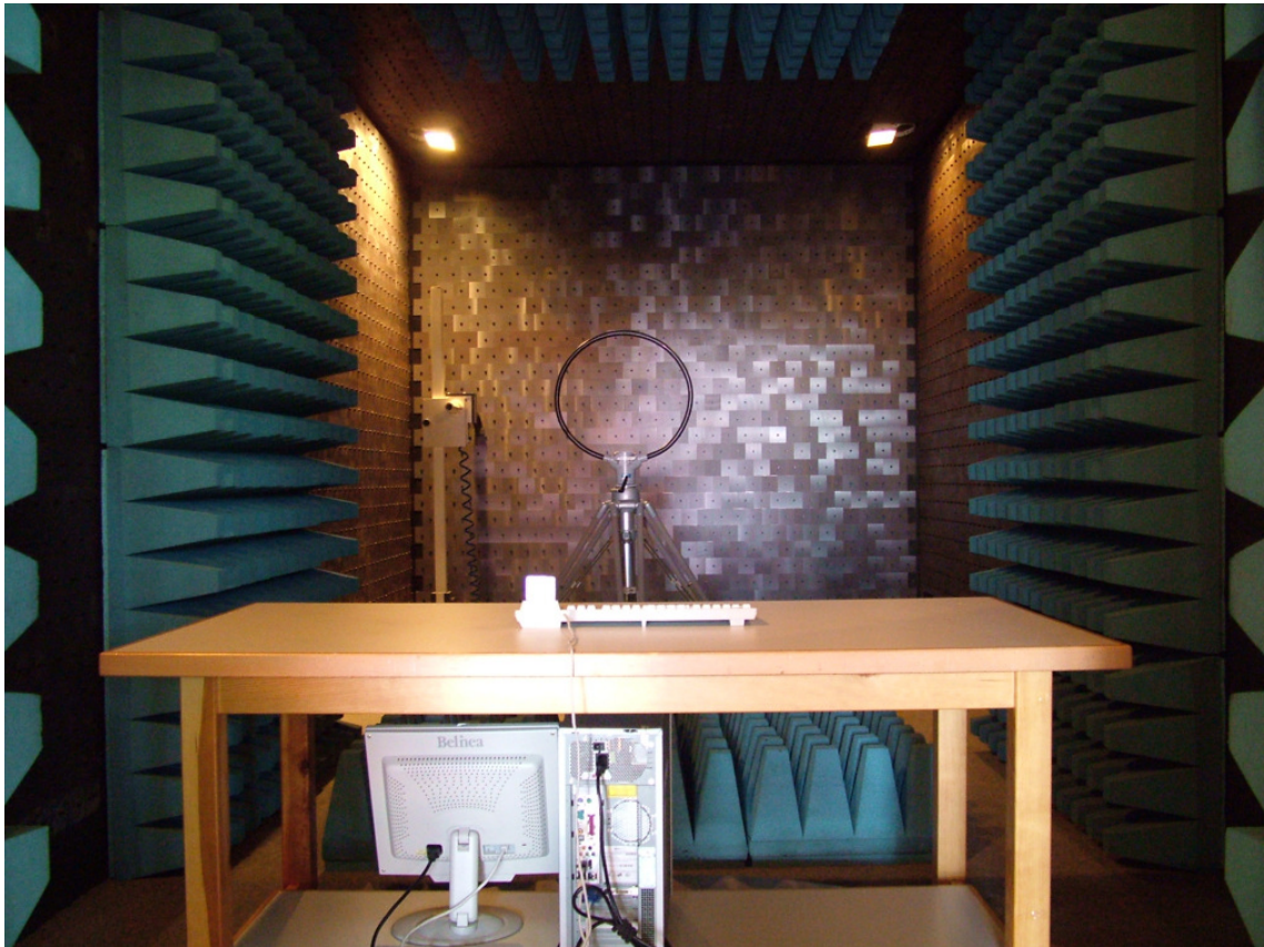
Picture 15-4: Occupied bandwidth test setup
