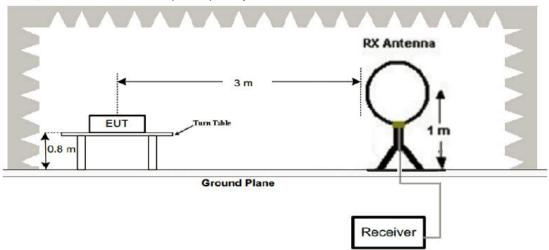
2. Radiated Emission Test-Up Frequency 30MHz~1GHz
