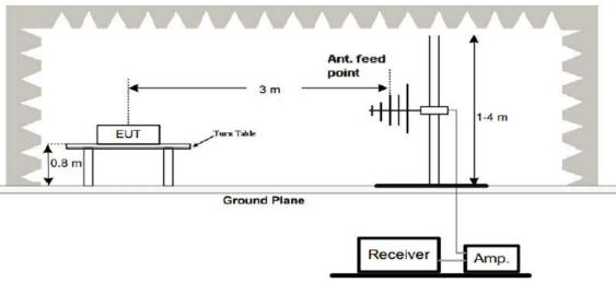
3. Radiated Emission Test-Up Frequency Above 1GHz
