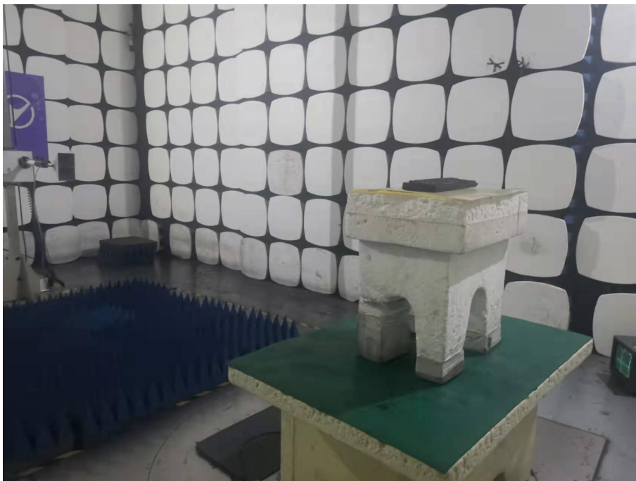
Spurious Emission Test Setup (Above 1GHz)
