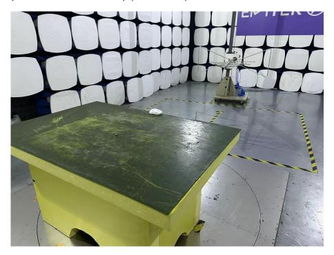
Spurious Emission Test Setup (Above 1GHz)
