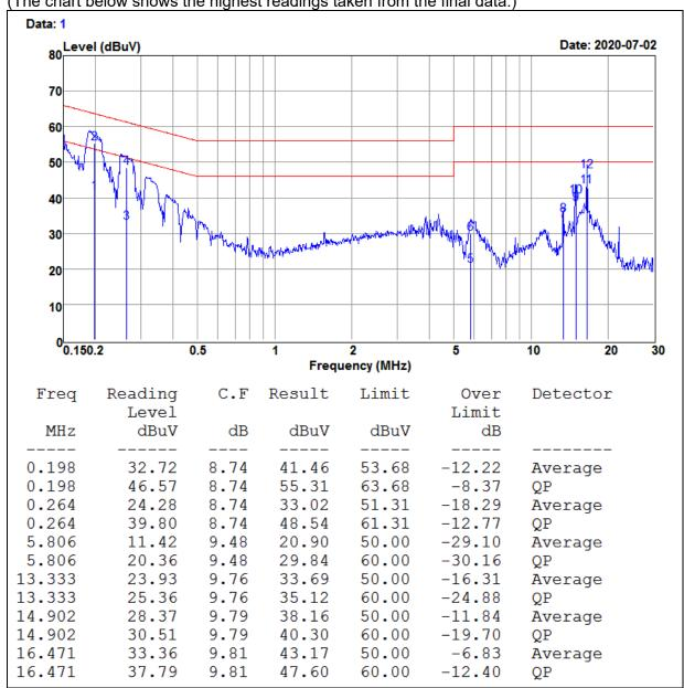
REMARKS: 1. Level (dBuV) = Read Level (dBuV) + LISN Factor (dB) + Cable Loss (dB)
