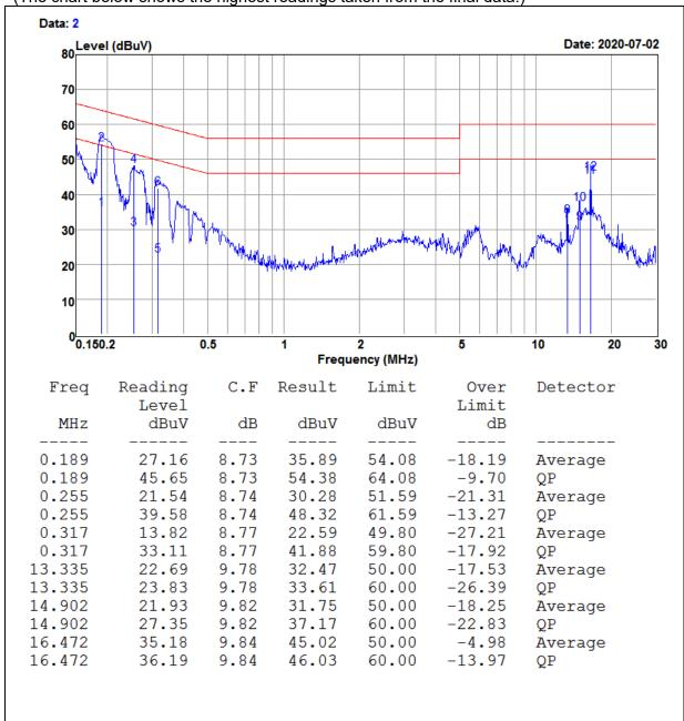
REMARKS: 1. Level (dBuV) = Read Level (dBuV) + LISN Factor (dB) + Cable Loss (dB)
