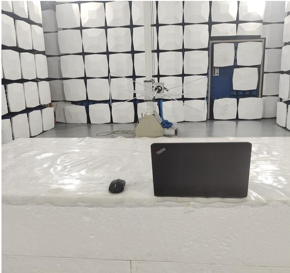
Radiated Emission Test Setup:
