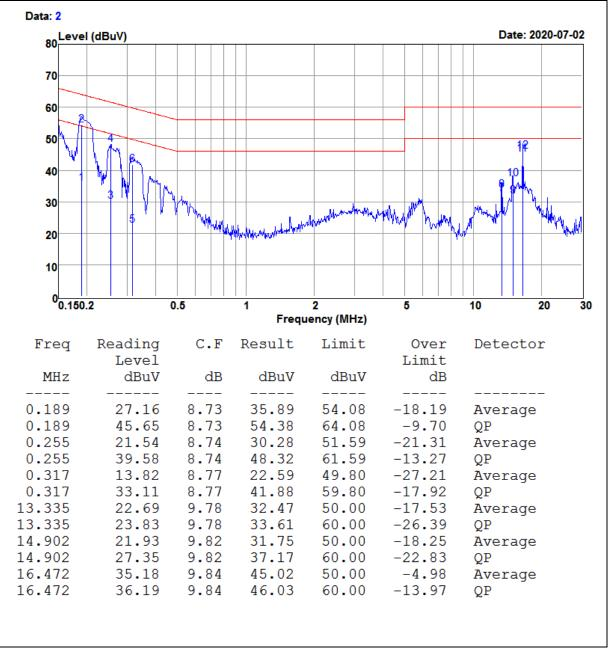
REMARKS : 1. Level (dBuV) = Read Level (dBuV) + LISN Factor (dB) + Cable Loss (dB) 2. Over Limit (dBuV) = Measured Level (dBuV) – Limits (dBuV)
