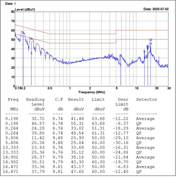
REMARKS : 1. Level (dBuV) = Read Level (dBuV) + LISN Factor (dB) + Cable Loss (dB) 2. Over Limit (dBuV) = Measured Level (dBuV) – Limits (dBuV)
