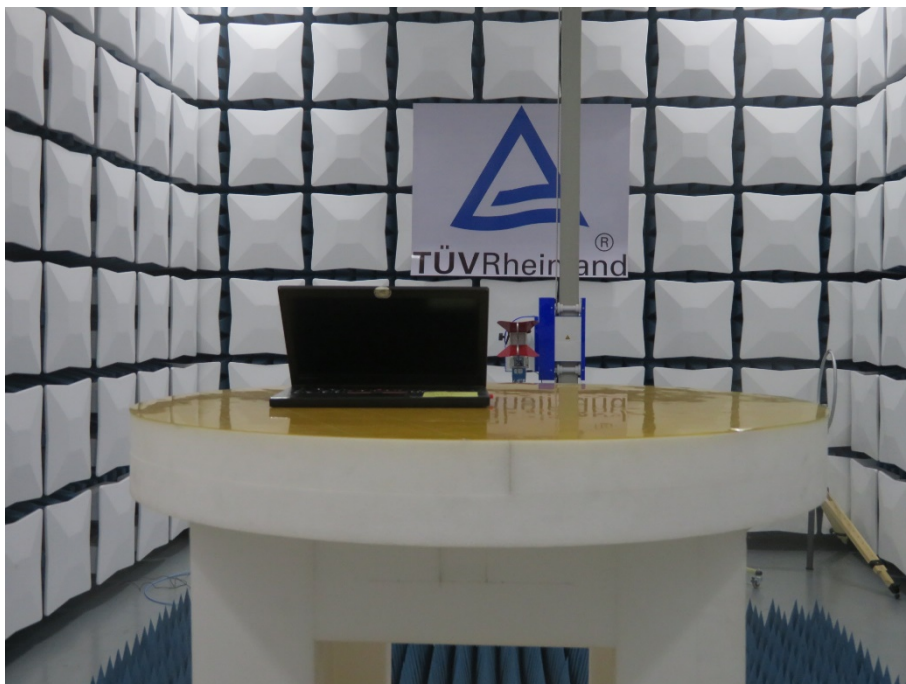
Photograph 2: Set-up for Radiated Spurious Emission, Above 1GHz
