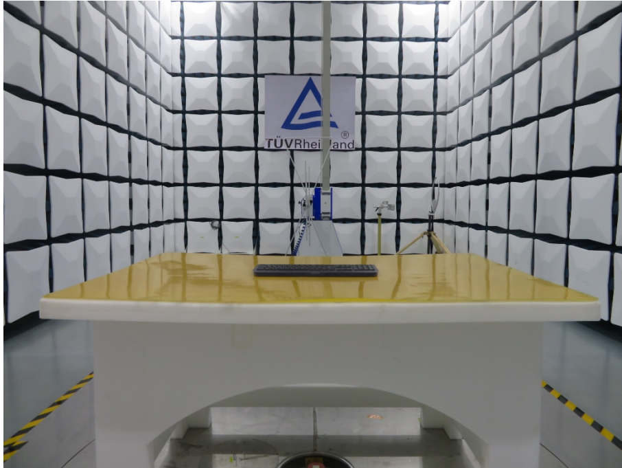
Photograph 2: Set-up for Radiated Spurious Emission, above 1GHz
