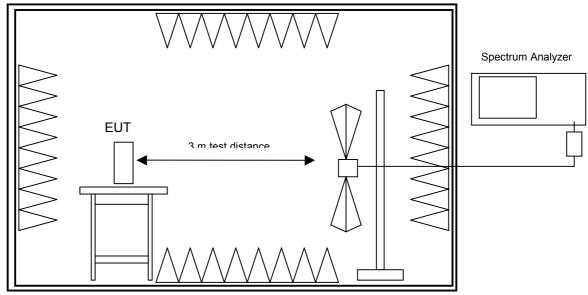
Fully anechoic chamber
