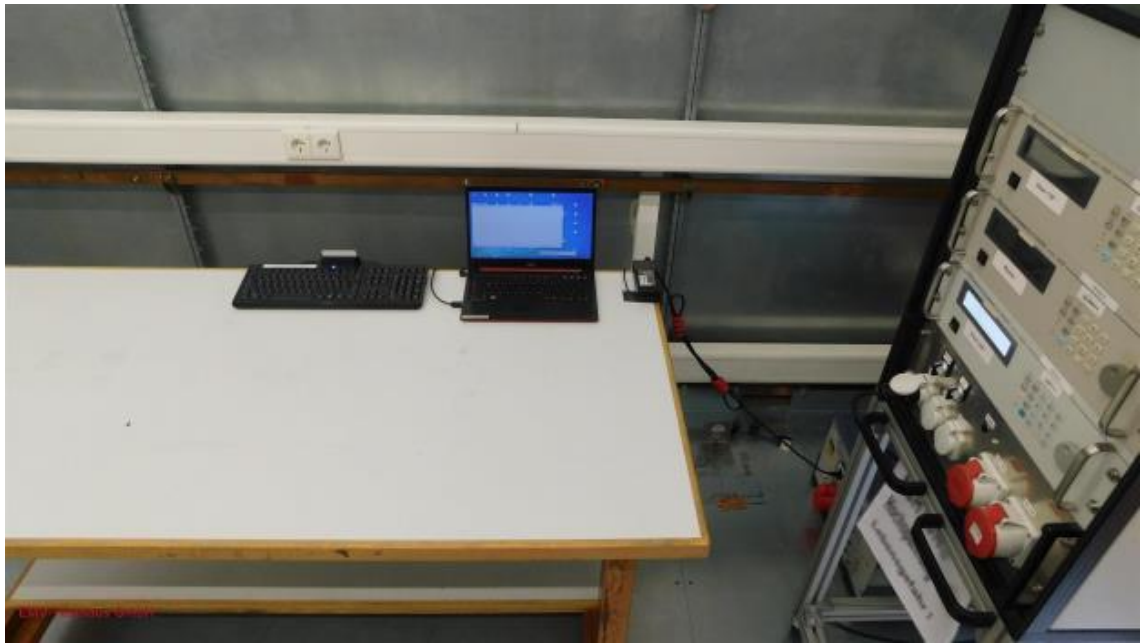
Picture 5: Test setup AC power line conducted emissions (front view)
