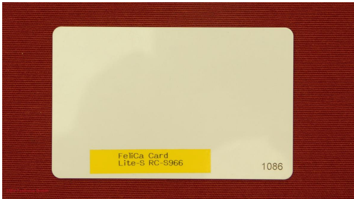
Picture 4: RFID tag 13.56 MHz
