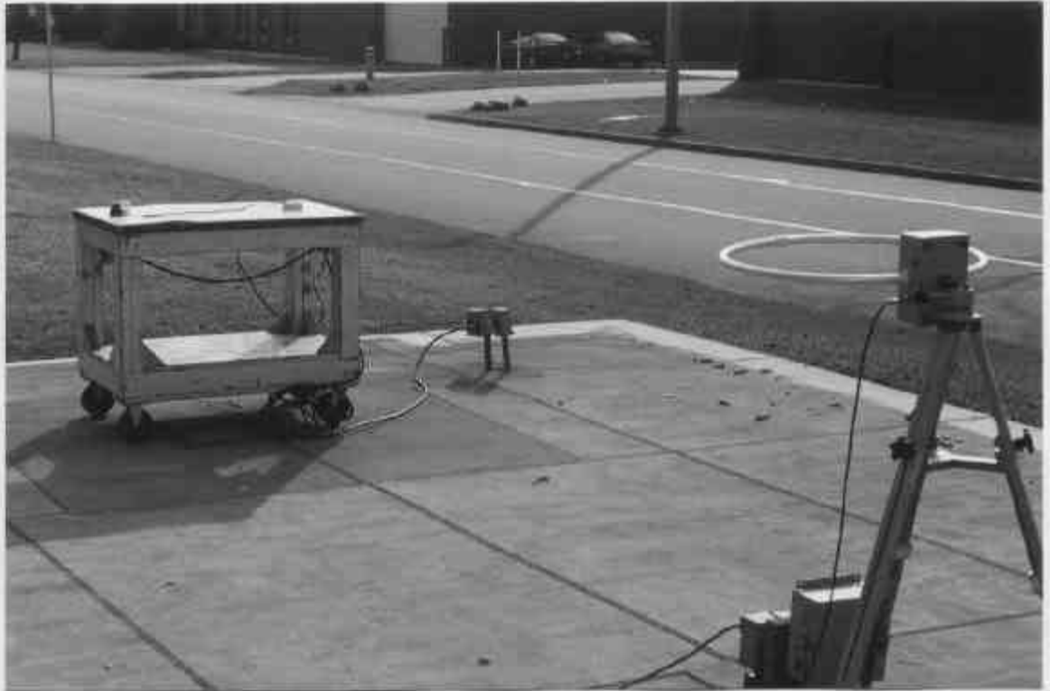
TEST SETUP FOR RADIATED EMISSIONS MEASUREMENTS MAXIMIZED FOR MEASUREMENT OF WORST CASE EMISSIONS HORIZONTAL POLARIZATION
