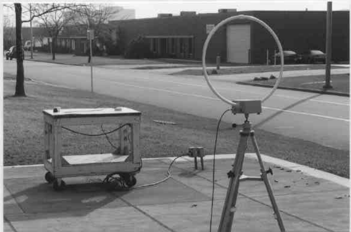
TEST SETUP FOR RADIATED EMISSIONS MEASUREMENTS MAXIMIZED FOR MEASUREMENT OF WORST CASE EMISSIONS VERTICAL POLARIZATION
