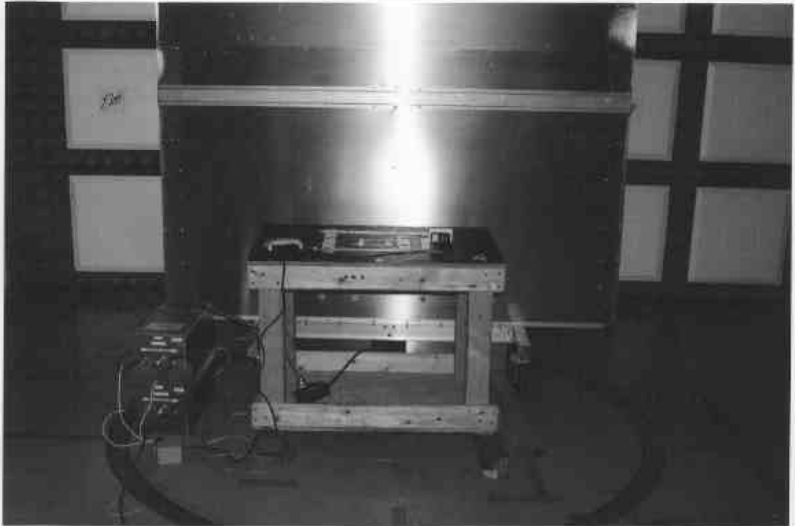
TEST SETUP FOR CONDUCTED EMISSIONS MEASUREMENT MAXIMIZED FOR MEASUREMENT OF WORST CASE EMISSIONS
