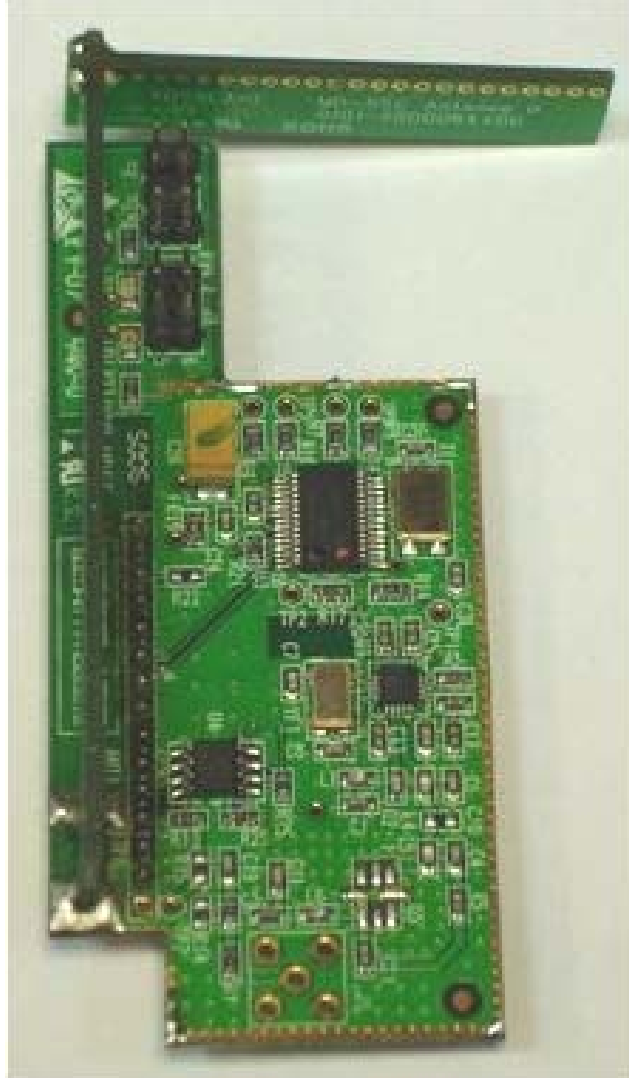
Photograph No.8 RF PCB without shielding
