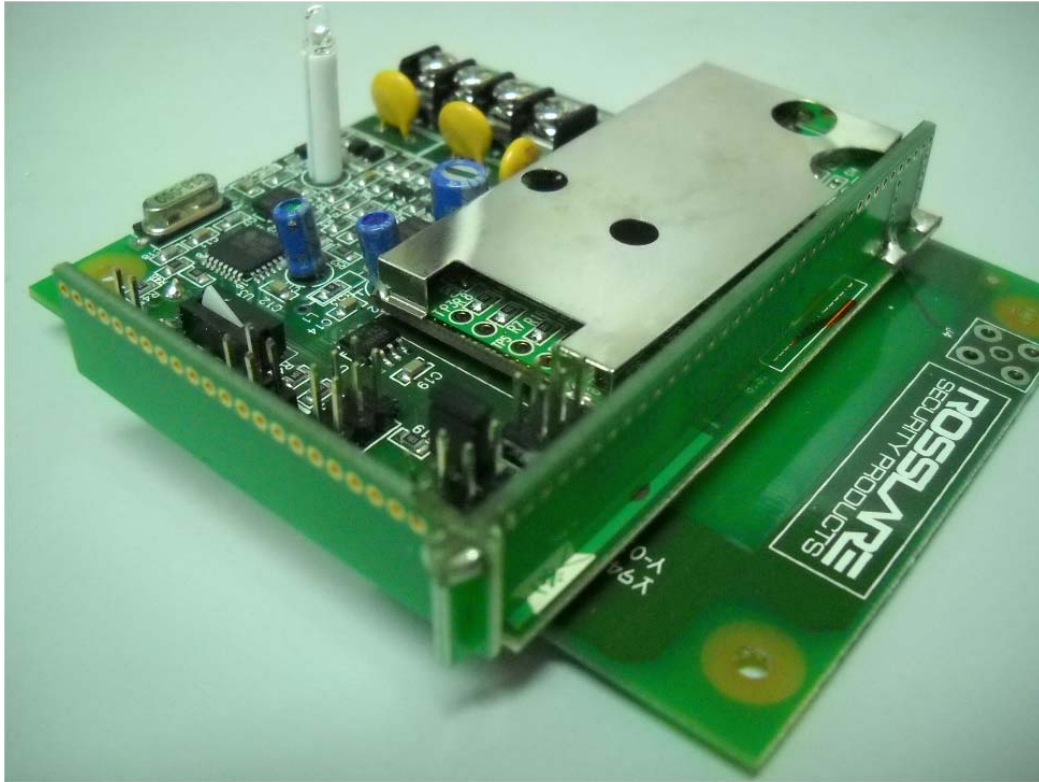
Photograph No.5 XR-16AG PCBs side view
