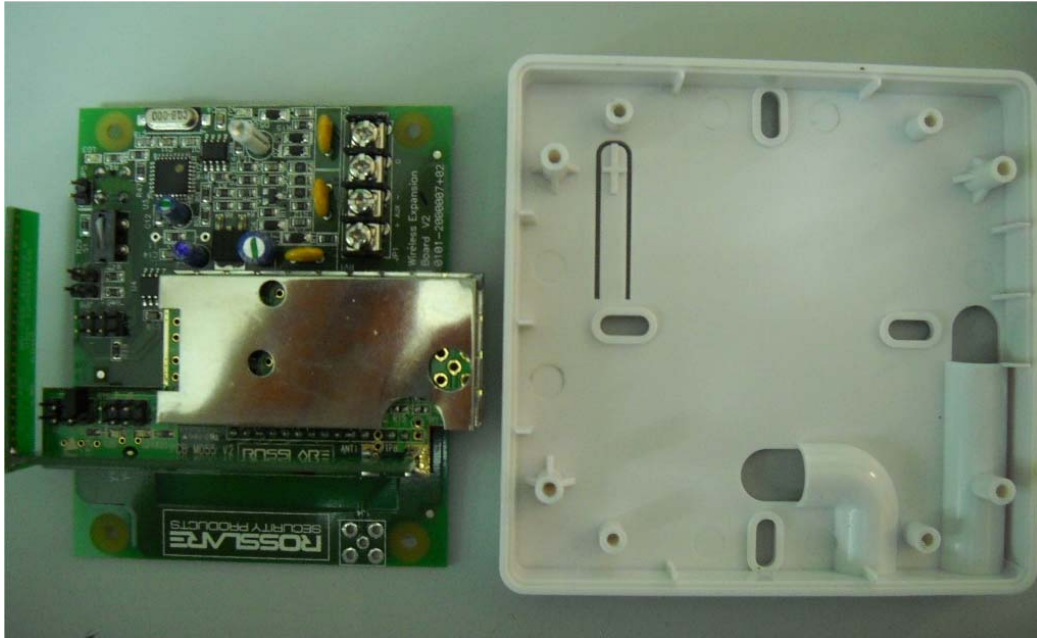
Photograph No.2 XR-16AG wireless expansion internal view
