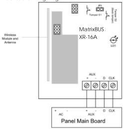
**NOTE:** Wiring must be done when the AuraSys™ L-4/6 panel power is turned off.
