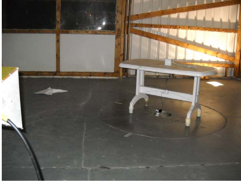
Photograph No.5 Setup for spurious emission measurements at the OATS above 1000 MHz
