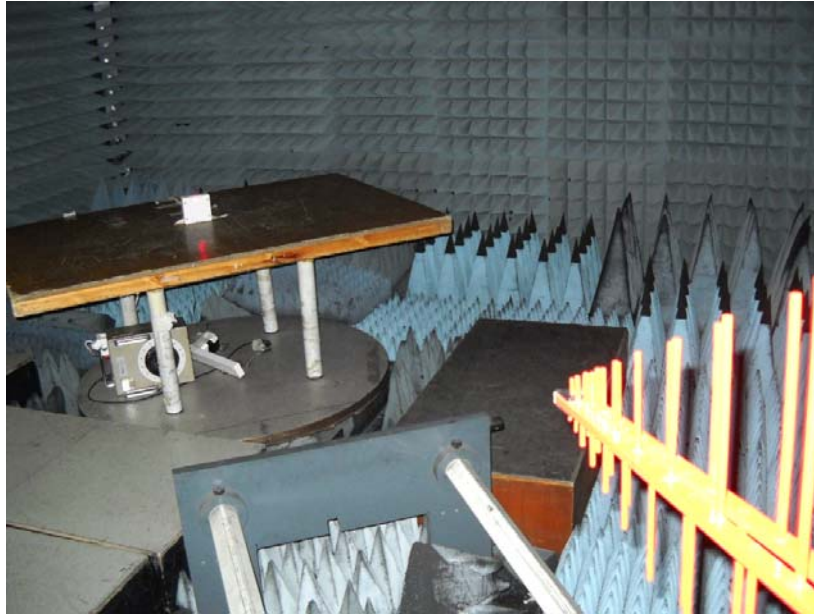
Photograph No.7 Setup for occupied bandwidth and periodic operation measurements
