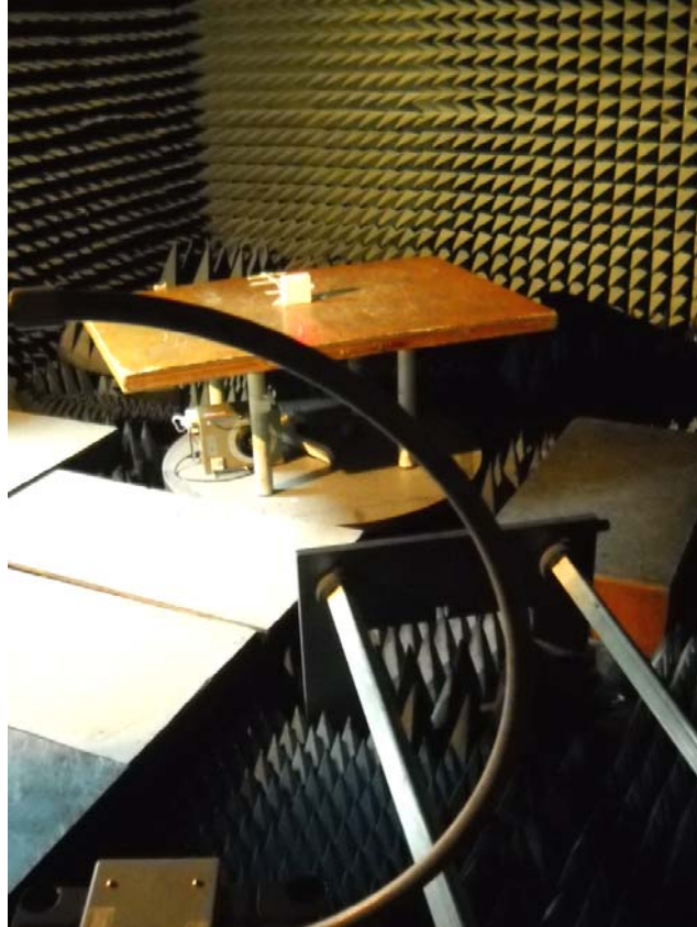
Photograph No.1 Setup for spurious emission measurements in the anechoic chamber below 30 MHz
