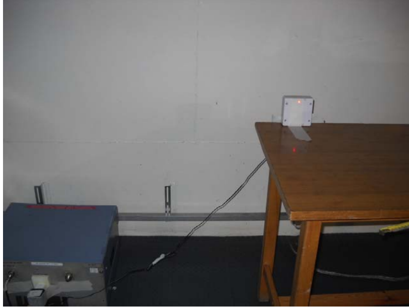
Photograph No.8 Setup for conducted emission measurements
