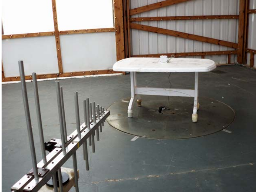
Photograph No.4 Setup for fundamental emission measurements at the OATS from 30 to 1000 MHz
