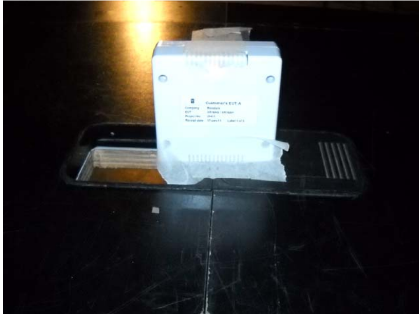
Photograph No.3 Setup for spurious emission measurements in the anechoic chamber, EUT close view
