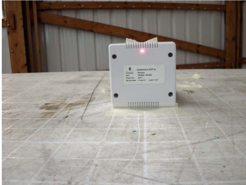
Photograph No.6 Setup for radiated emission measurements at the OATS, EUT close view
