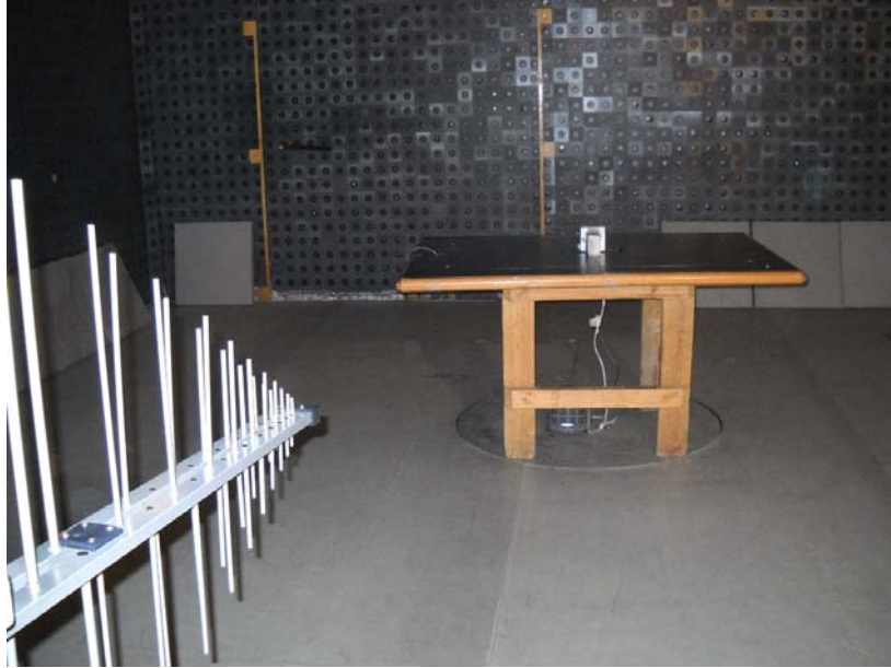
Photograph No.2 Setup for spurious emission measurements in the anechoic chamber from 30 to 1000 MHz
