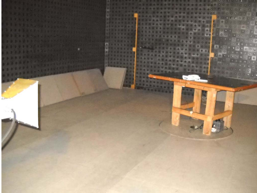
Photograph No.3 Setup for spurious emission measurements in the anechoic chamber above 1 GHz
