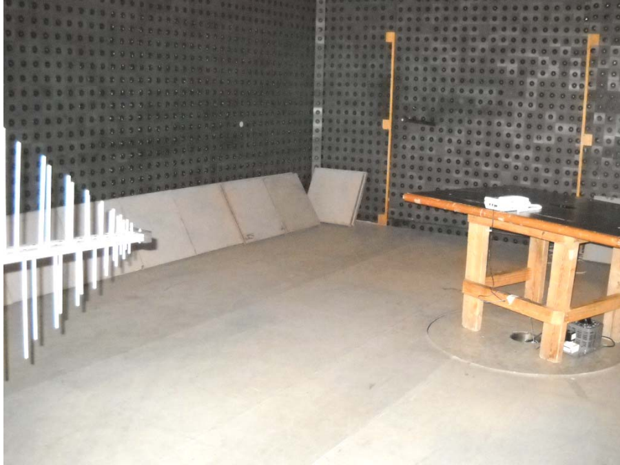
Photograph No.2 Setup for spurious emission and occupied bandwidth measurements in the anechoic chamber in 30 - 1000 MHz range
