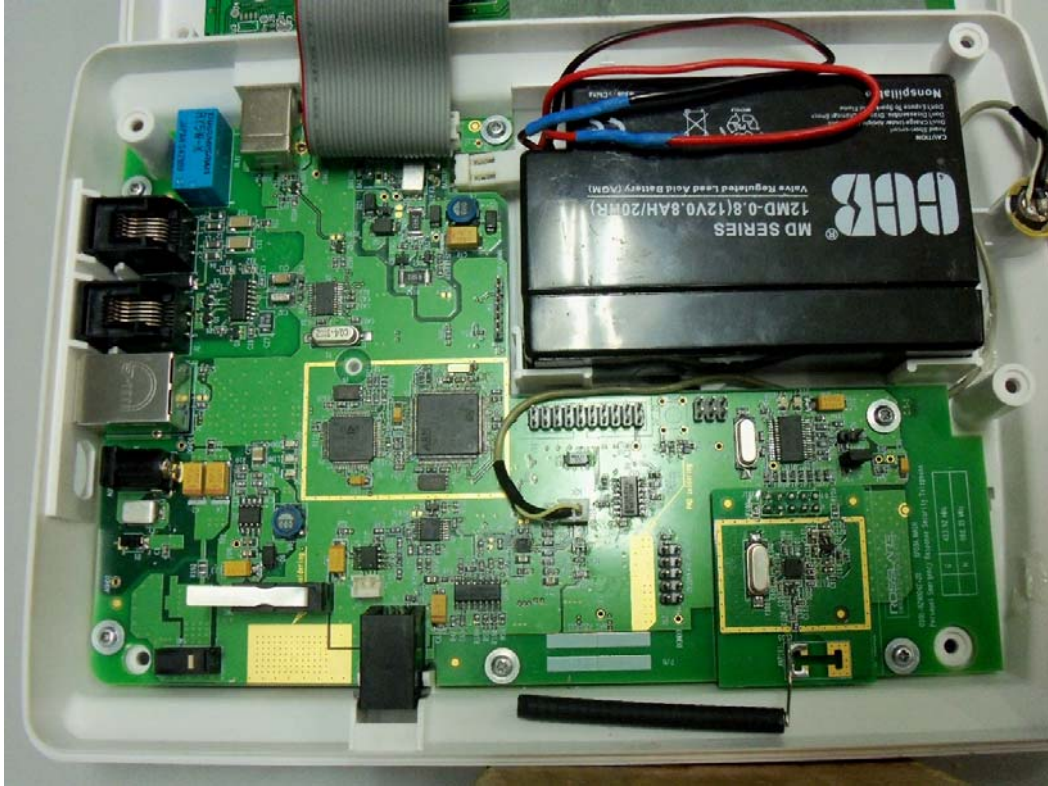
Photograph No.1 Wireless Elderly Assist SP-03V2G internal view (case)
