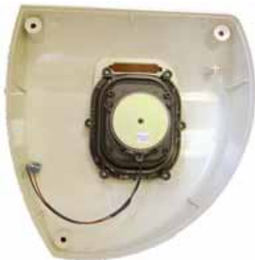
Figure 1: Cover with Loudspeaker
