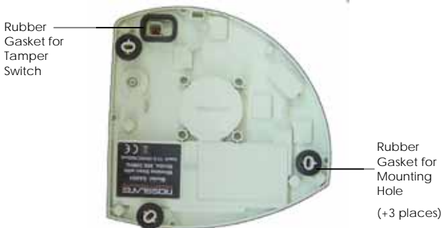
Figure 5: Base with Sealing Gaskets
