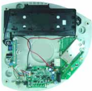
Figure 2: Base with PCBs
