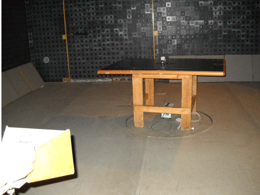
Photograph No.3 Setup for radiated emission measurements in the anechoic chamber above 1000 MHz
