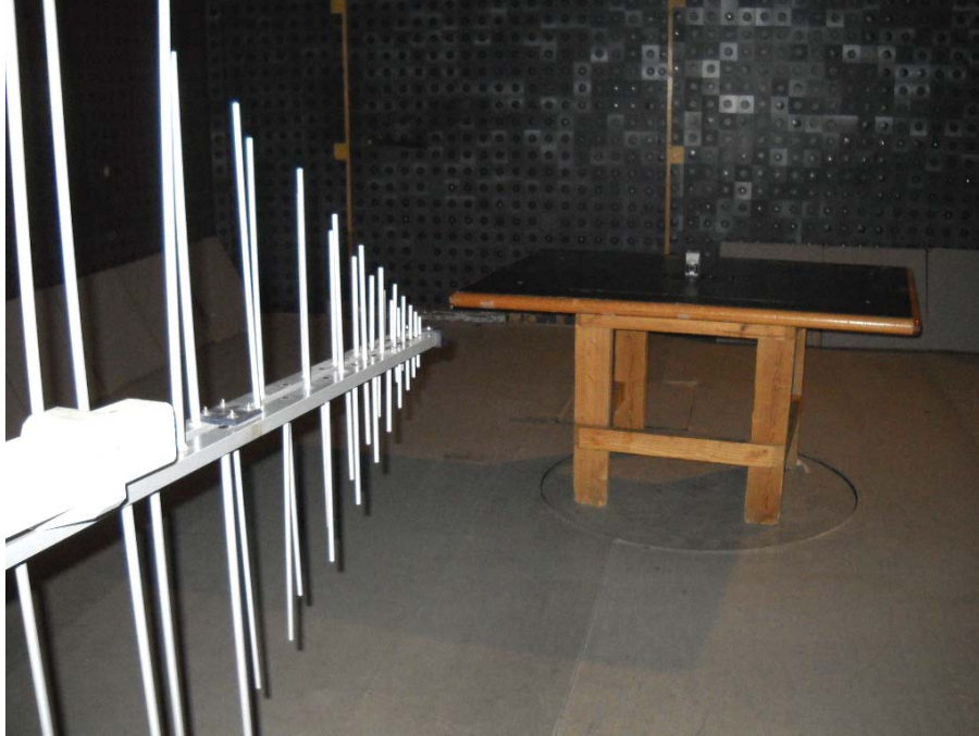
Photograph No.2 Setup for radiated emission measurements in the anechoic chamber from 30 to 1000 MHz
