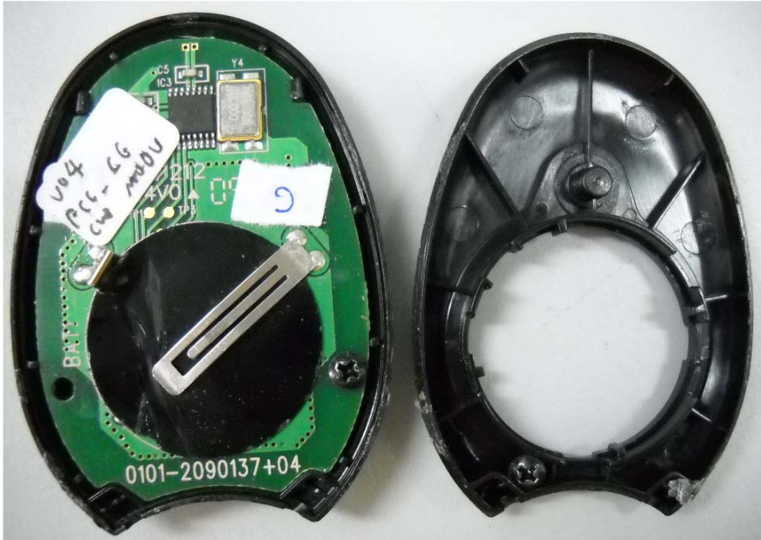
Photograph No.3 SA-33G remote control internal view
