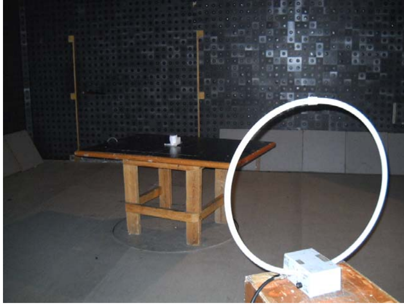
Photograph No.1 Setup for spurious emission measurements in the anechoic chamber below 30 MHz
