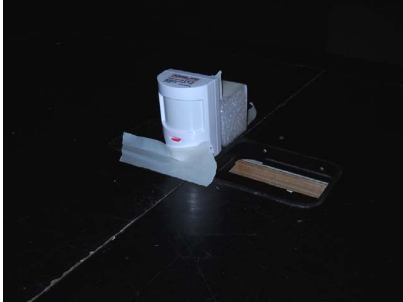
Photograph No.3 Setup for radiated emission measurements in the anechoic chamber, EUT close view
