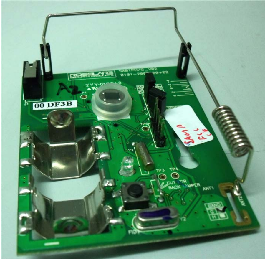
Photograph No.6 Antenna close view
