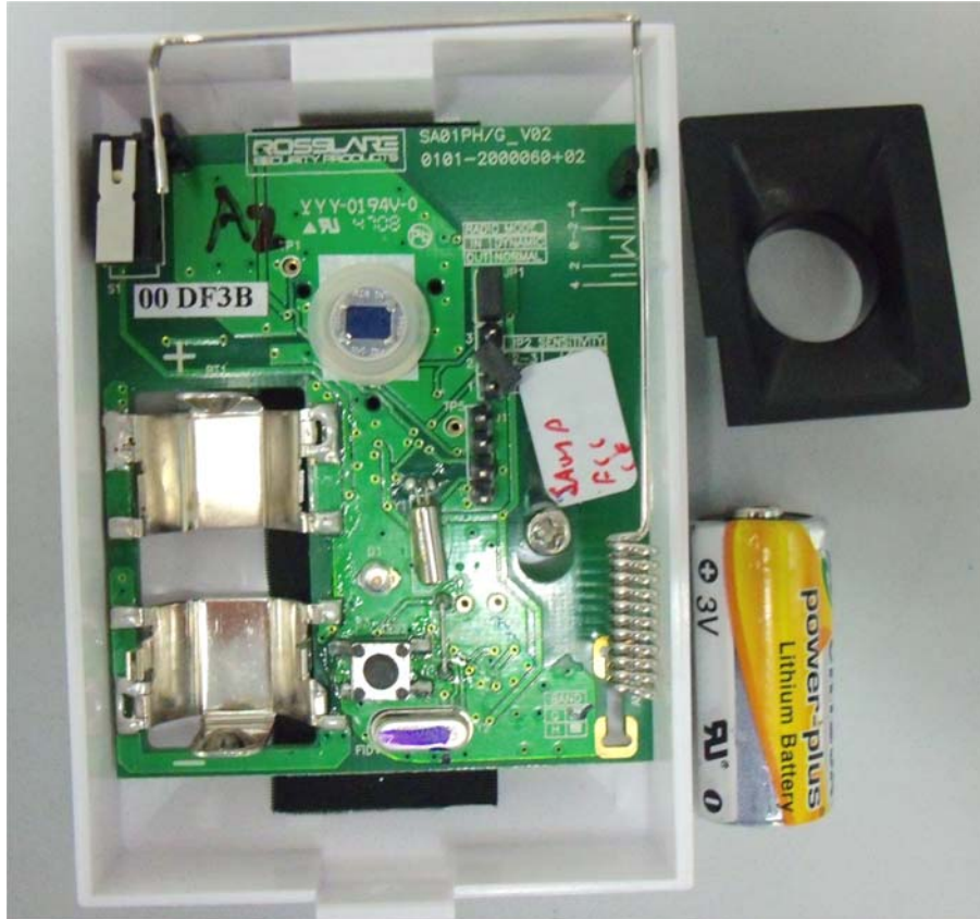
Photograph No.2 SA-01PG PIR detector internal view
