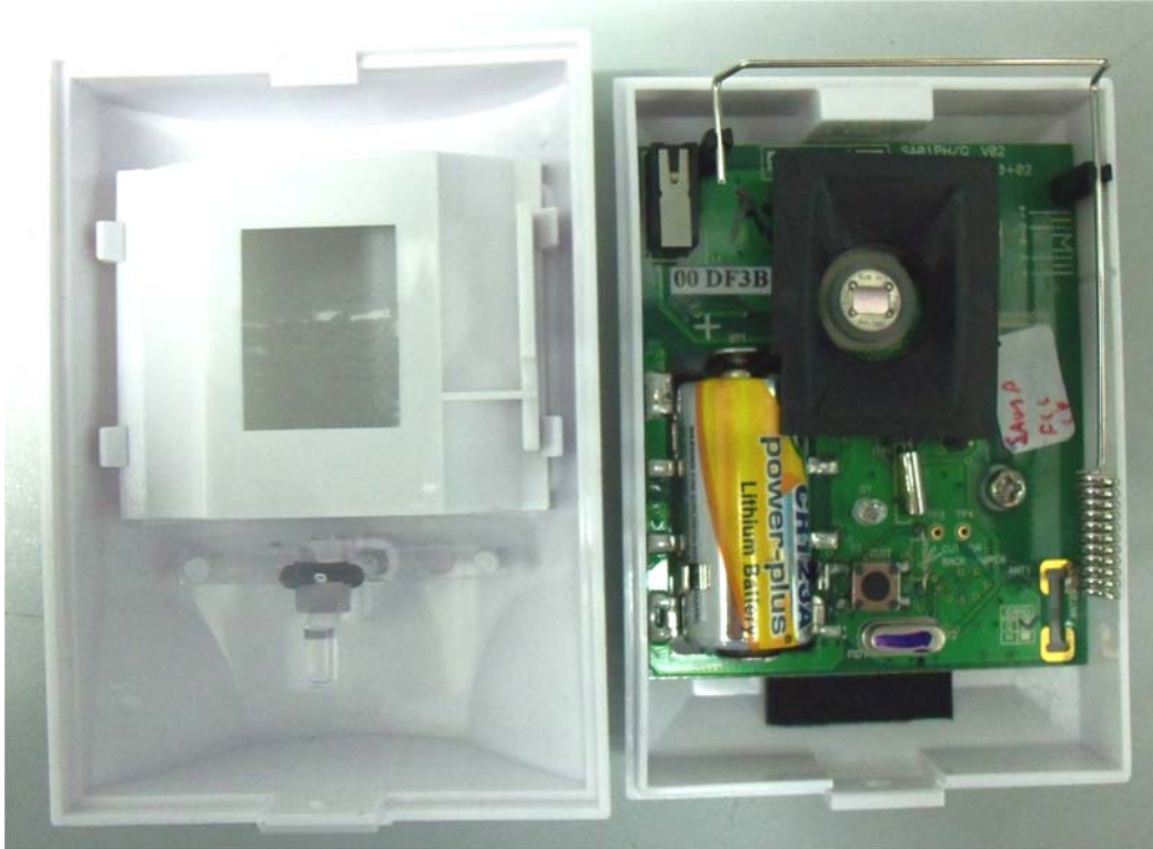
Photograph No.1 SA-01PG PIR detector internal view
