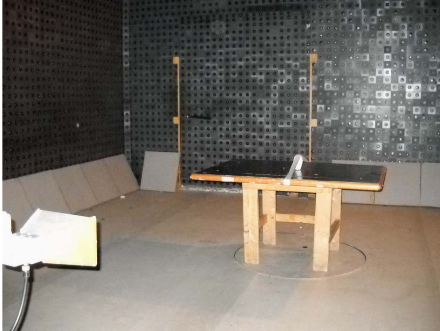
Photograph No.4 Setup for spurious emission measurements in the anechoic chamber above 1000 GHz
