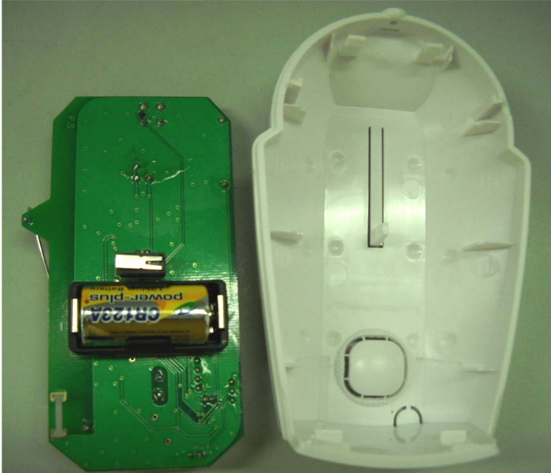
Photograph No.2 PYR-2011AG detector internal view
