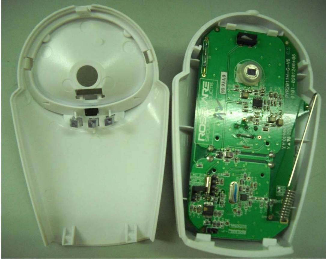
Photograph No.1 PYR-2011AG detector internal view
