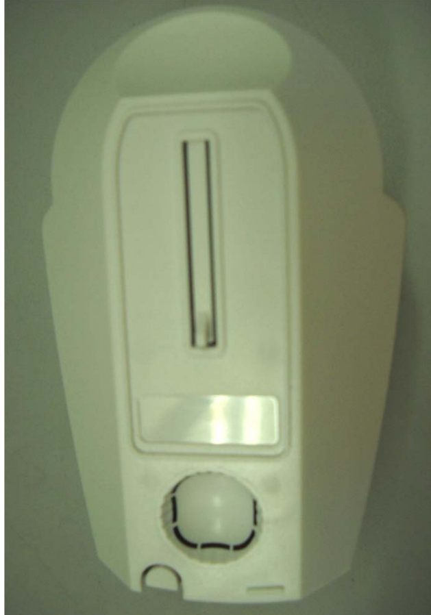
Photograph No.2 PYR-2011AG PIR detector rear side view
