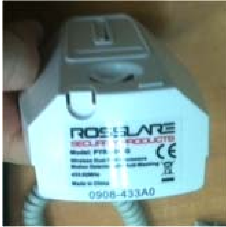
Photograph No.3 PYR-2011AG PIR detector bottom view
