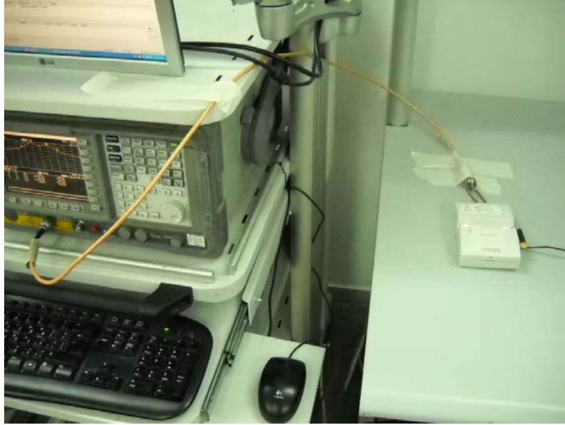
Photograph No.6 Setup for occupied bandwidth measurements
