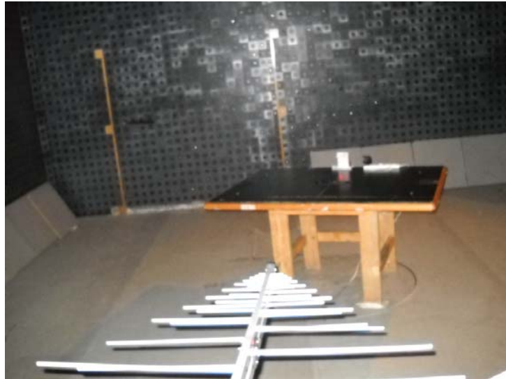
Photograph 8.2.2 Setup for radiated emission measurements, EUT cabling
