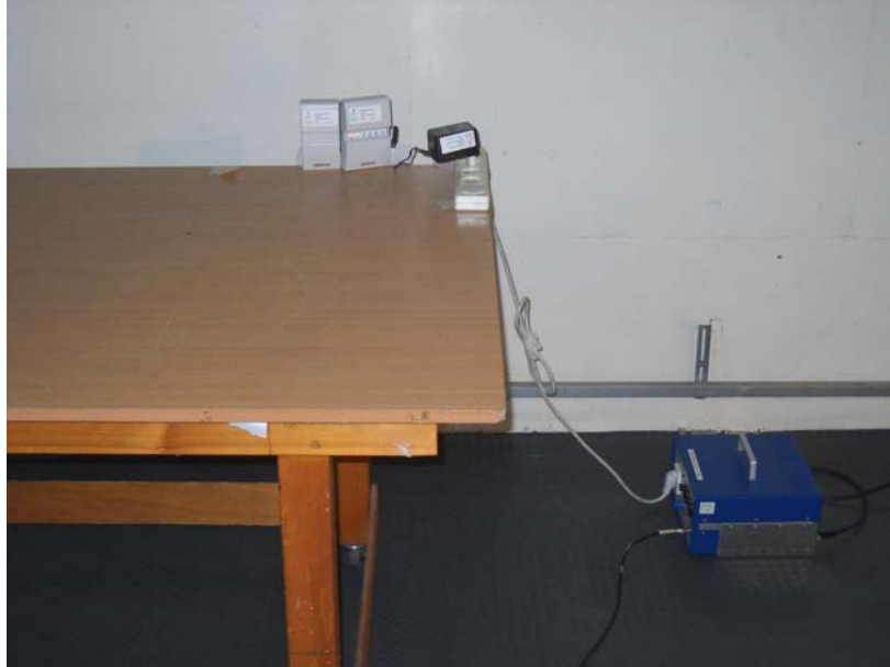
Photograph No.6 Setup for conducted emission measurements on AC power lines
