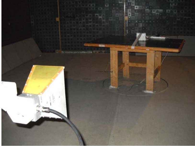
Photograph No.3 Setup for spurious emission measurements in the anechoic chamber above 1000 GHz
