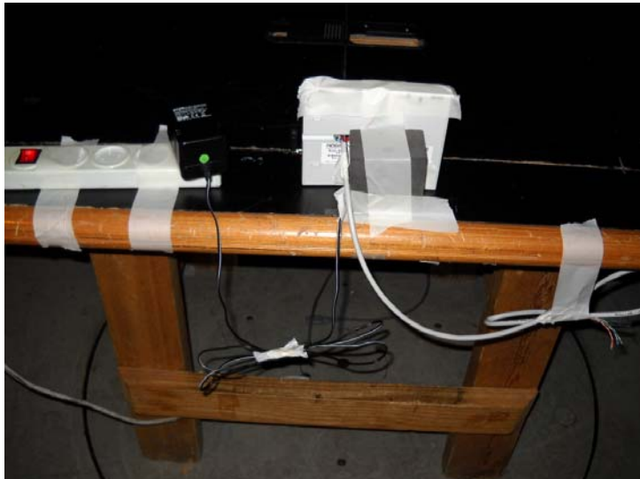
Photograph 8.2.2 Setup for radiated emission measurements, EUT cabling
