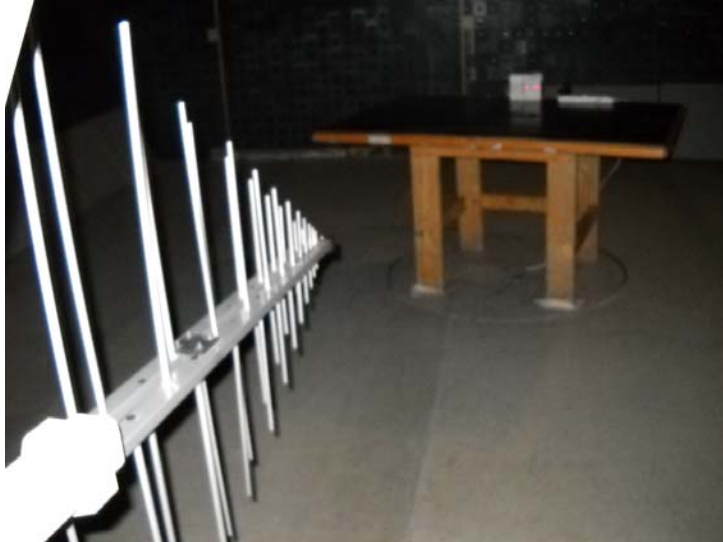
Photograph 8.2.2 Setup for radiated emission measurements, EUT cabling
