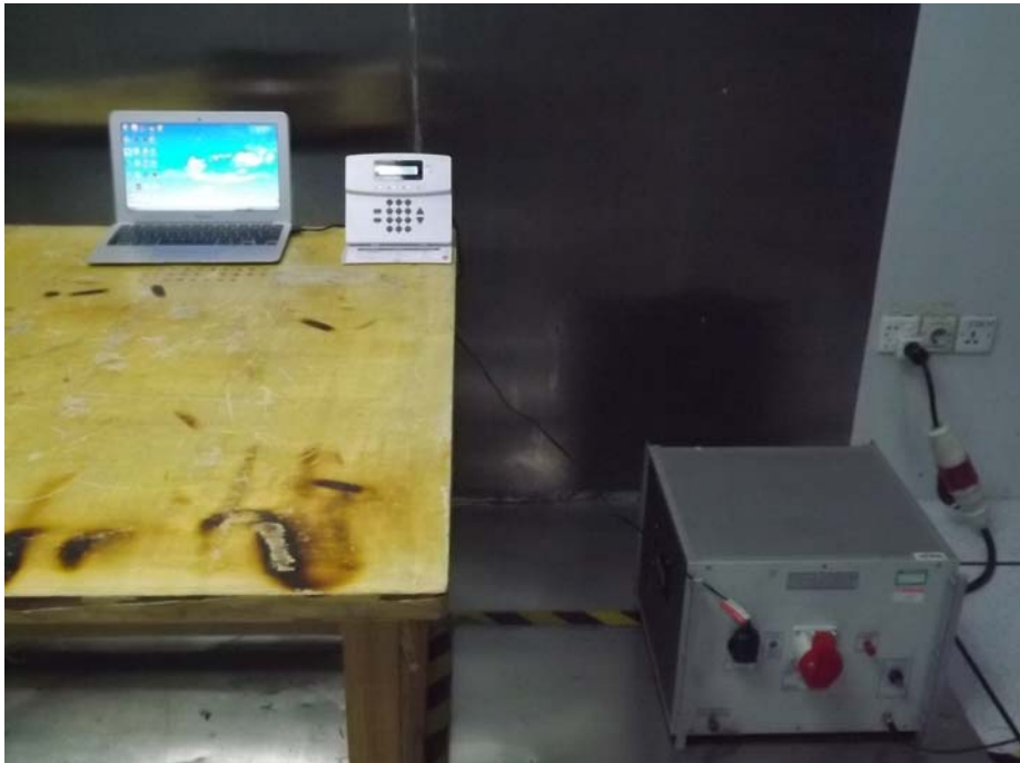
Conducted Disturbance at Mains Terminal Test Setup
