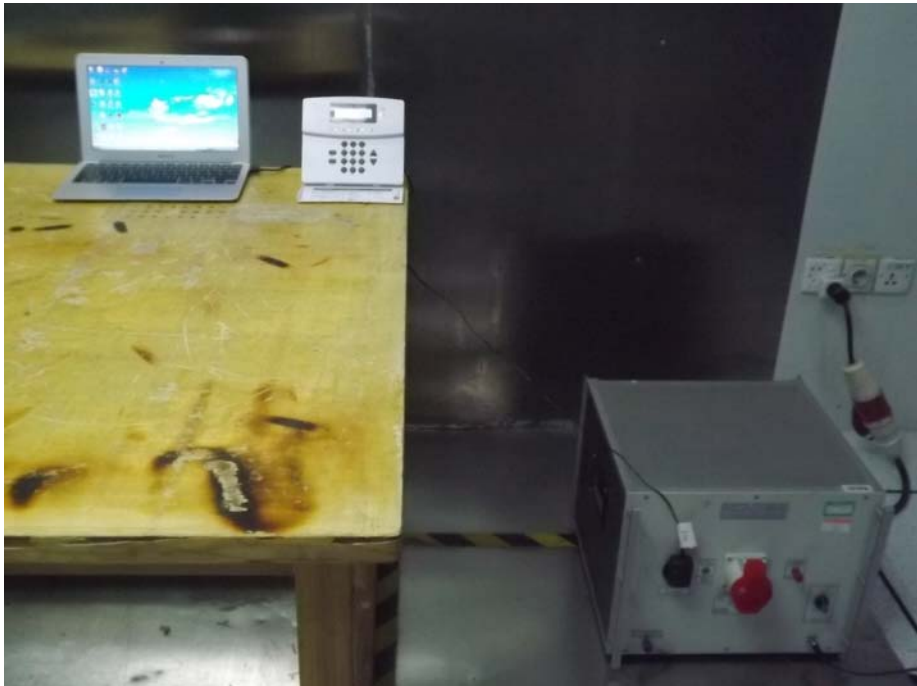
Conducted Disturbance at Mains Terminal Test Setup
