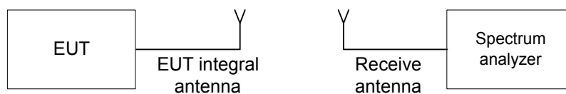
Figure 7.1.1 Setup for transmitter shut down test
