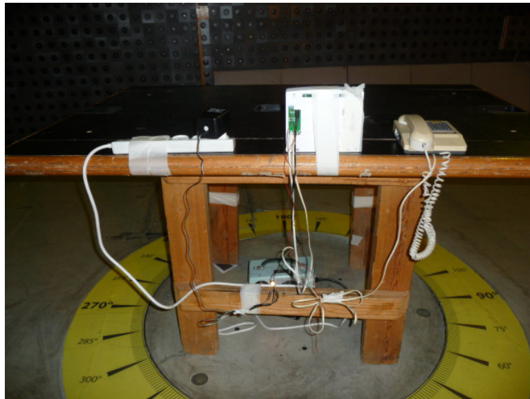
Photograph 8.2.3 Setup for final radiated emission measurements, EUT cabling
