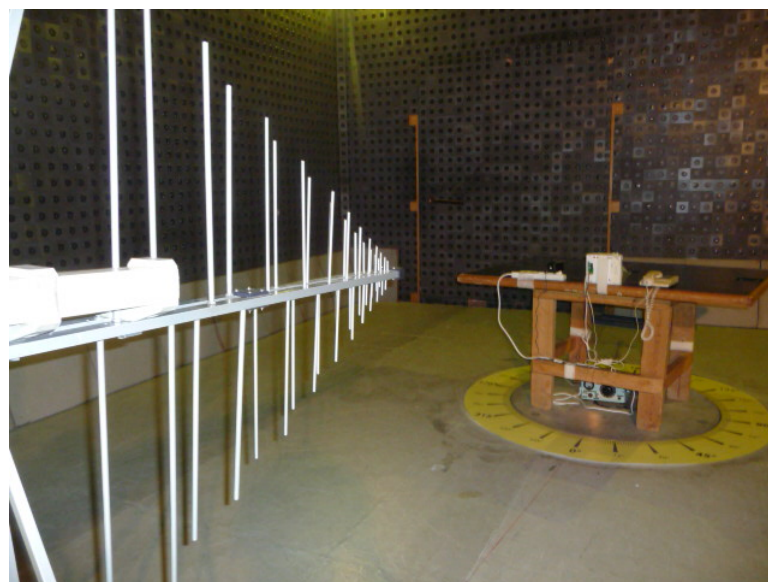
Photograph 8.2.1 Setup for final radiated emission measurements, general view
