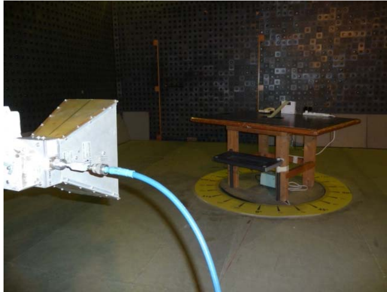
Photograph 8.2.2 Setup for spurious emission field strength measurements above 1000 MHz
