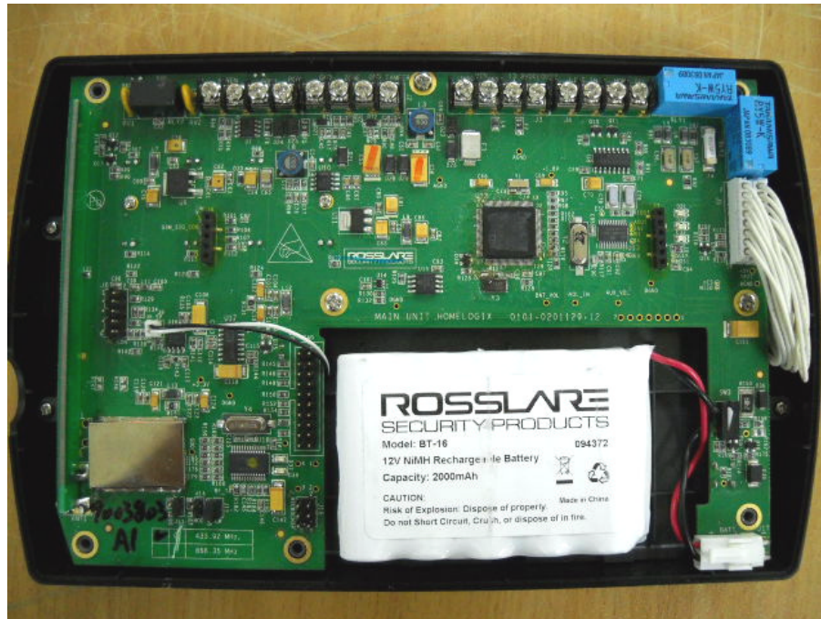
Photograph No.2 HLX-40BGE wireless security panel internal view
