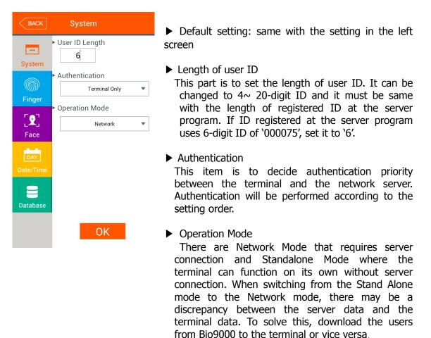
To apply the setting value, press [OK] button or press [BACK] button to cancel and to move to the upper menu. If [OK] button is pressed without changing the setting value, directly move to upper menu.
