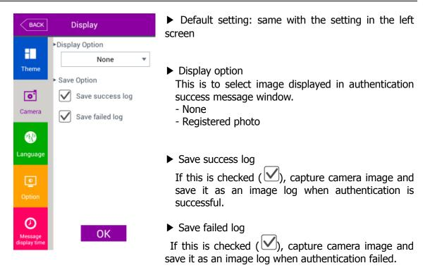
To apply the setting value, press [OK] button or press [BACK] button to cancel and to move to the upper menu.
