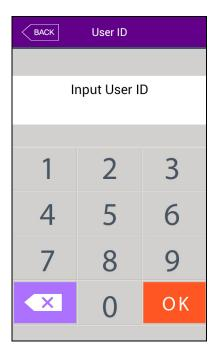
Input user ID and press **[OK]** button to display fingerprint input, face input, card input or password input screen according to Authentication Method of a user.
