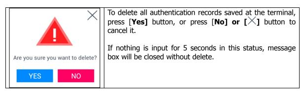
Success message will be displayed when successfully deleted by pressing **[Yes]**. All authentication logs including image log will be deleted. They can't be recovered after **deleting**.
