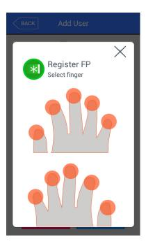
① Press [Fingerprint] button in [Add user] screen to register.
