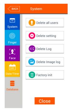
To delete all users, press **[Delete all users]** button. To reset the setting value, press **[Delete setting]** button. To reset authentication record, press **[Delete Log]** button. To delete only image log, press **[Delete image log]** button. To delete the whole data to make the device to factory setting status, press **[Factory Init]** button.
