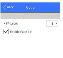
'Fingerprint verification level' (Default setting: '0') This item is to decide fingerprint verification level for each user. Authentication level for each registered user can be changed by change this value.
