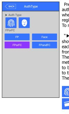
Press [**Auth Type**] button in **[Add user**] screen to set authentication method. (However, this can be set only when more than one authentication method are registered.)
