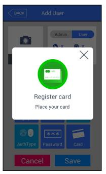
Press **[Card]** button in **[Add user]** screen to register a card. To move out without registering, press  $[\times]$  button.
