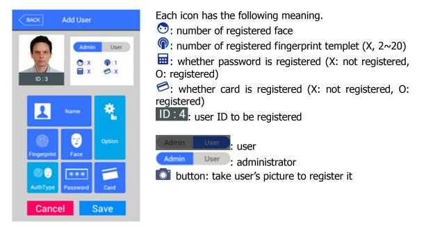
Press **[name]** to register name, press **[Fingerprint]** to register fingerprint, press **[face]** to register face, press **[card]** to register card, press **[password]** button to register password. Basically, everybody is registered as a user. Press **[administrator]** button to convert into an administrator. **To save registration after completing,** press **[Save] button** or press **[Cancel]** or **[BACK]** button to cancel input or to move out of it.
