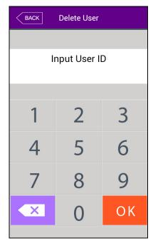
Input user ID to be deleted and press [**OK**] button. Press [BACK] button to cancel and move out.
